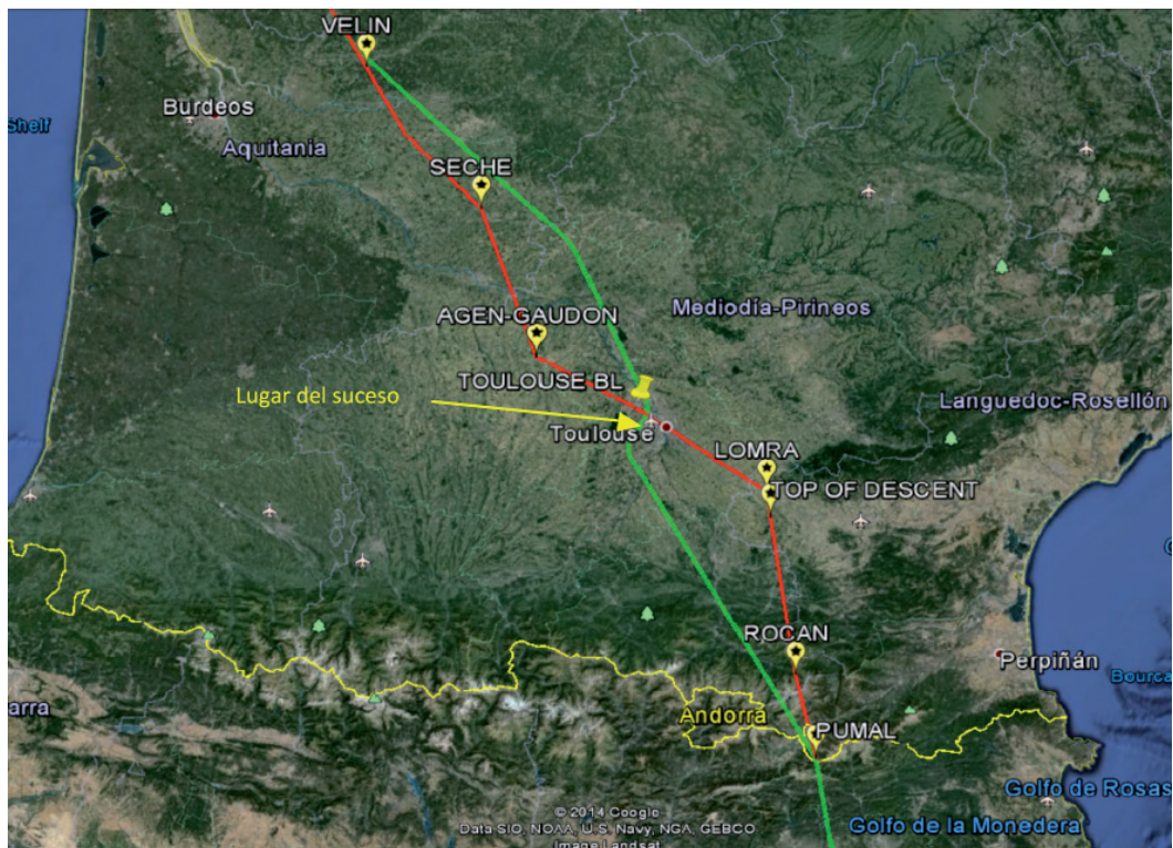
Figure 6. The flight path as per the operational flight path is shown in red and the actual path taken in green
