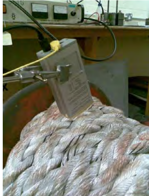
Figure 4 – Arrangement for measuring charge decay time from the rope.
