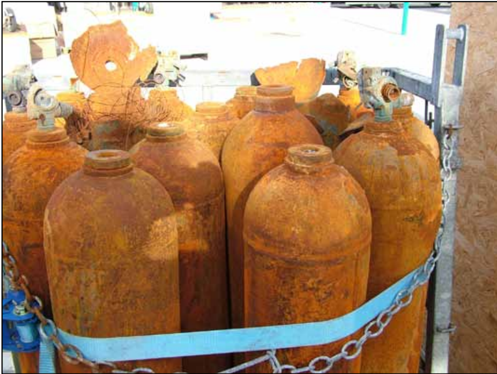
Explosion damaged acetylene bottles
