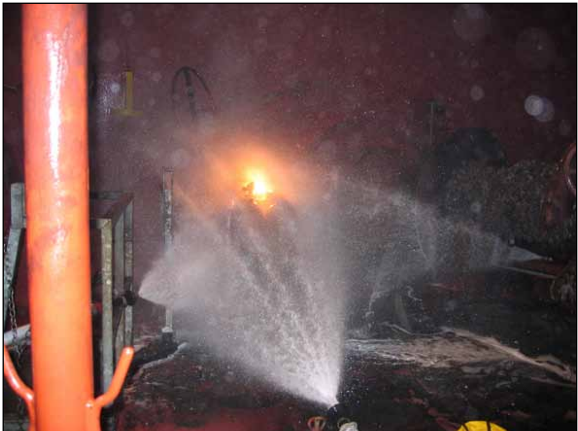
Hoses rigged to cool down the acetylene and oxygen bottles
