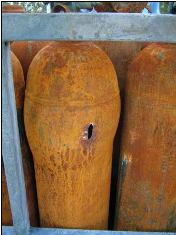
Distorted acetylene bottles
