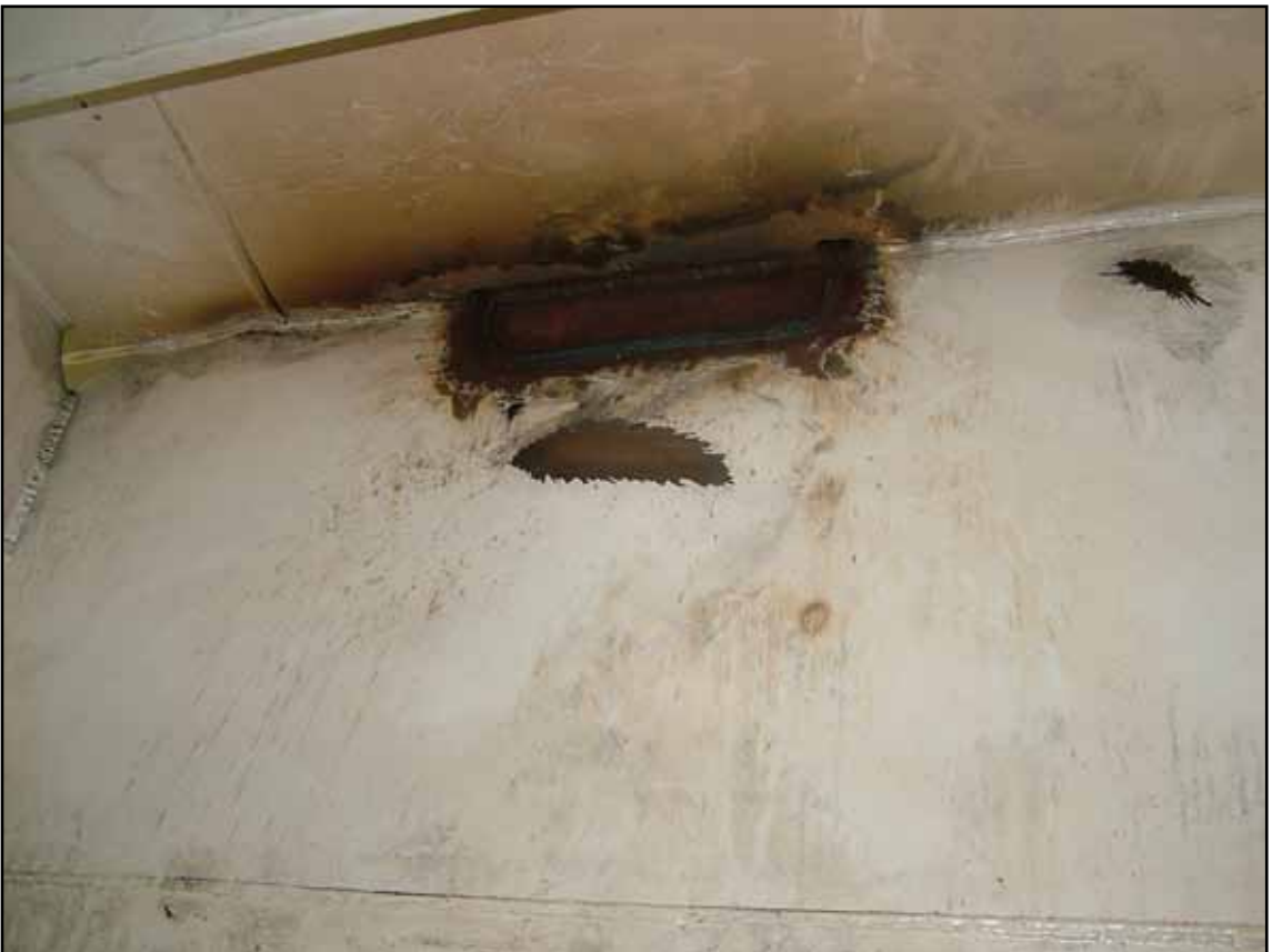
Hull indentations - port side bow thruster room
