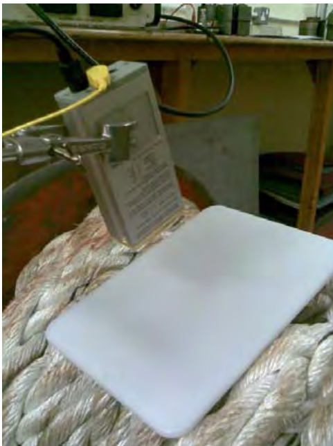
Figure 5 – Arrangement for measuring charge decay time from an insulating plastic plate.
