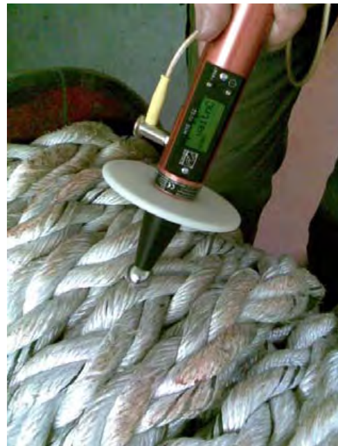
Figure 6 – Arrangement for measuring charge transfer in any discharges from the rope.
