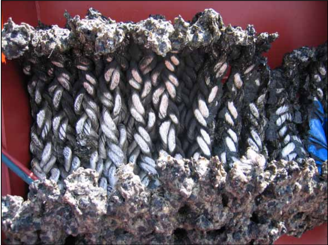
Fire damaged mooring rope from the port windlass winch drum
