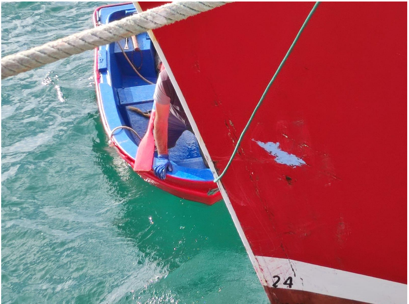
Figura 6. Close-up of the damage suffered by the ZERUKO ERREGIÑA during the accident
