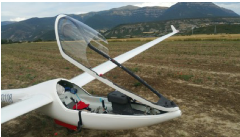
Figure 1. Damage to the glider's canopy
