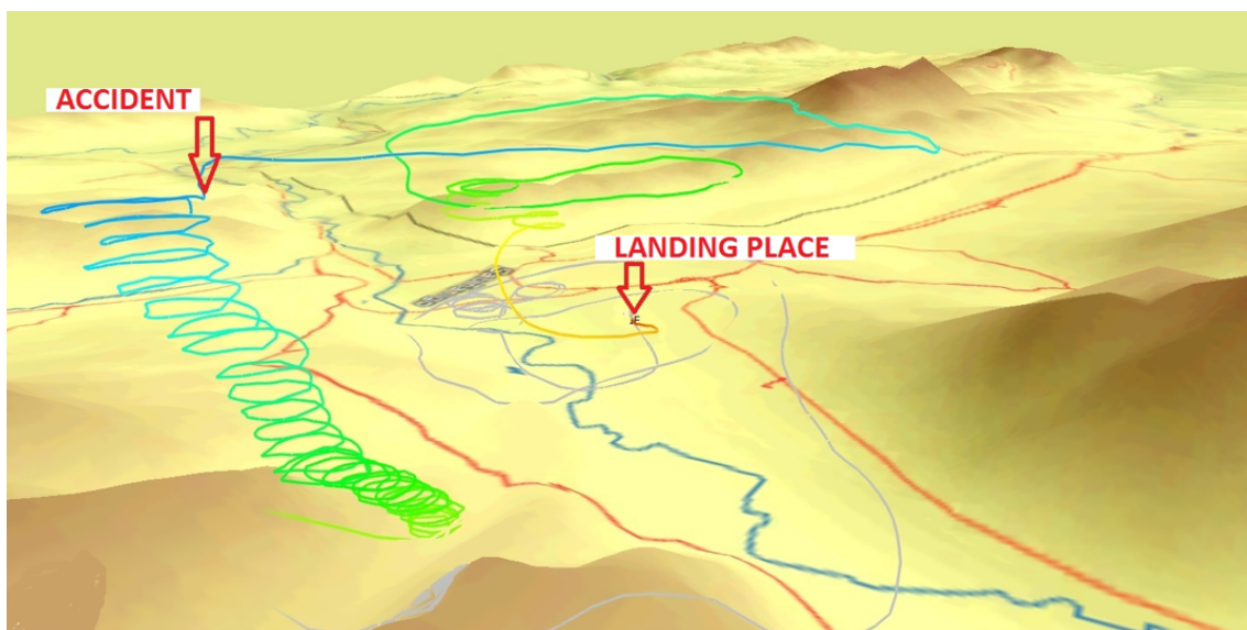
Figure 2. Views of the final climb showing where the aircraft impacted the vulture and the descent to the landing location
