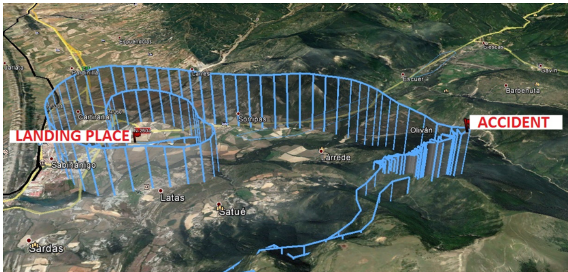
Figure 3. Views of the final climb showing where the aircraft impacted the vulture and the descent to the landing location
