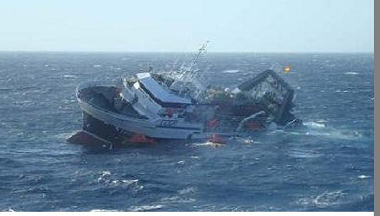
Trawler vessel MONTE GALIÑEIRO sank while it was operating 235 miles from Saint John's after an uncontrolled flood broke out inside her engine room. The origin of the flood could not be determined, but because the vessel sank quickly, it was determined that the flood must have occurred through the sea water collector; however, other hypotheses were not ruled out.
