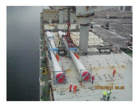
Wind Mill Blades being loaded on top of No. 4 & 5 Hatch Covers
