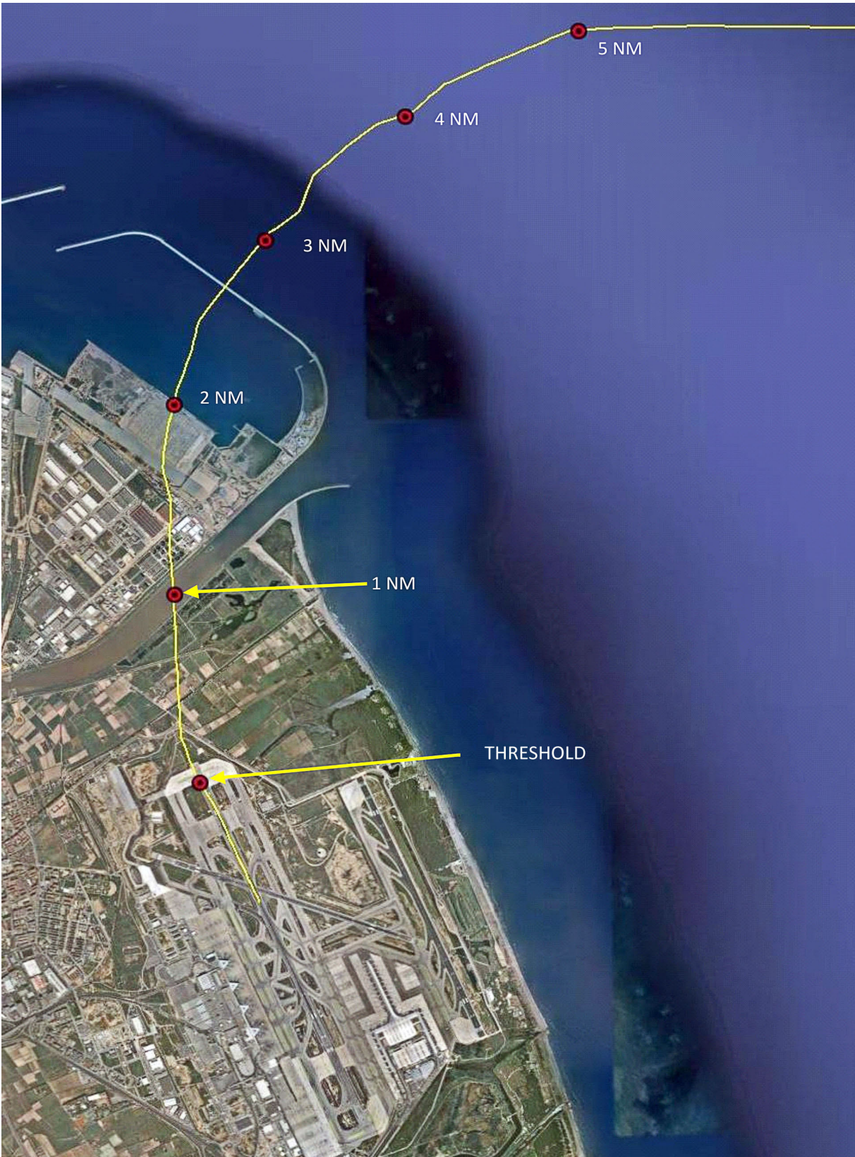
Figure 7. Top view of the last 5 NM of the aircraft's flight path. The distances shown are from the threshold and measured based on the aircraft's actual flight path
