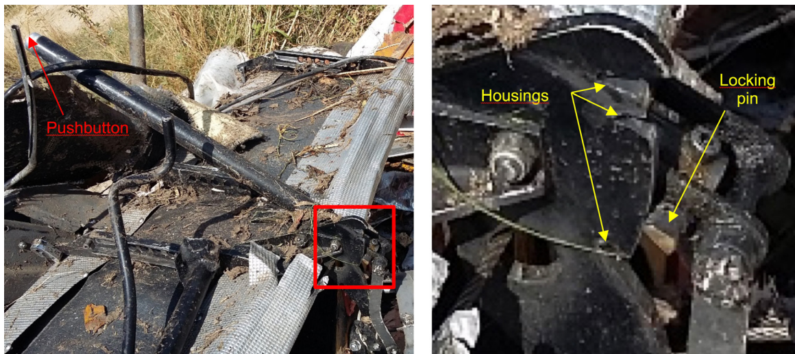
Figure 6. Photograph of the flap lever (left). At the right, close-up of the area shown in the red box in the figure on the left, providing a better view of the locking pin and the three control housings
