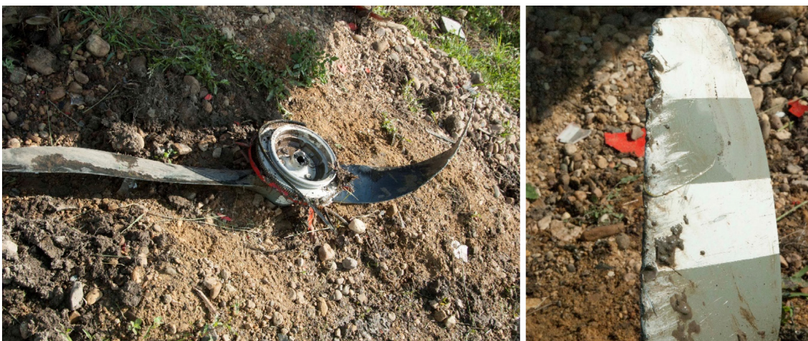
Figure 7. Photograph of the propeller (left) and close-up of the top surface of one of the blades (right)
