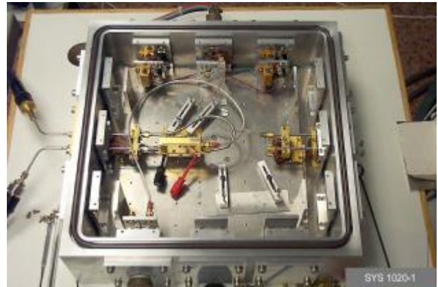
Figure 3 Low noise amplifier in the cryostat for gain fluctuation measurements.
